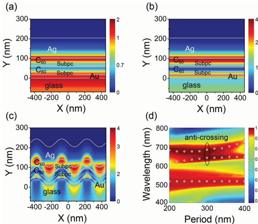
**Figure 4.** Distribution of the magnetic field intensity in the planar double-junction cells at the wavelengths of 510 nm (a), 650 nm (b), and the corrugated double-junction cells with period of 300 nm at the wavelength of 650 nm (c). (d) Dispersion relationship for the wavelength versus the period of the corrugation of the corrugated double-junction cells.
