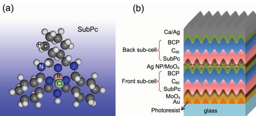
**Figure 1.** (a) Chemical structure of the donor material boron subphthalocyanine chloride. (b) Schematic structure of the corrugated double-junction solar cells.
