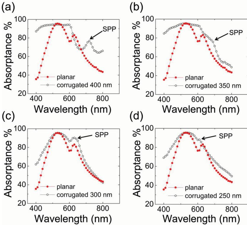
**Figure 3.** The experimentally measured absorption spectra of the planar and corrugated double-junction solar cells with periods of 400 nm (a), 350 nm (b), 300 nm (c) and 250 nm (d).
