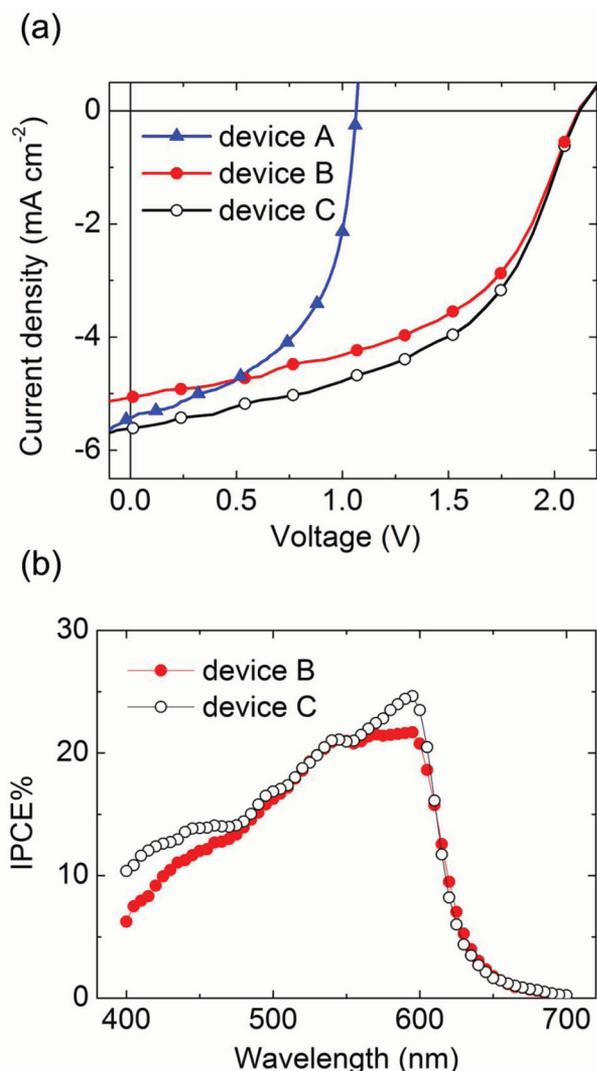
**Figure 5.** (a) J–V characteristics of the devices A, B, and C. (b) IPCE spectra of the planar (device B) and corrugated (device C) double-junction solar cells.
