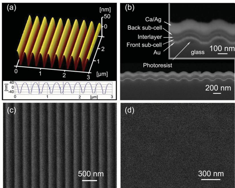
**Figure 2.** (a) Atomic force microscopy (AFM) image of the 1D corrugation on the photoresist surface, and the inset is the cross section. (b) SEM cross section of the corrugated device. (c,d) Top-view SEM images of the corrugated and planar double-junction solar cells, respectively.
